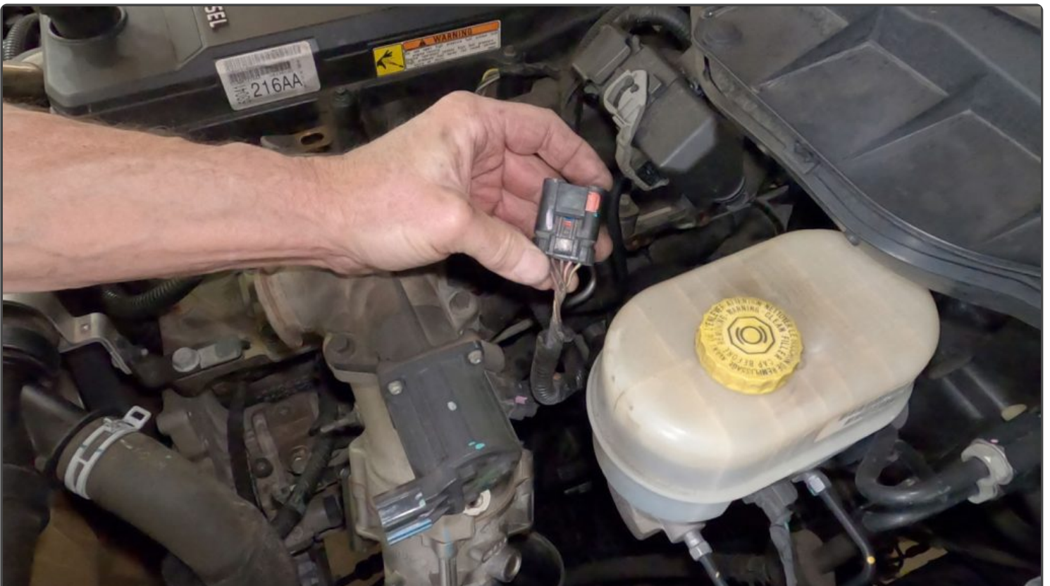
MAP Sensor and throttle body connector location.
